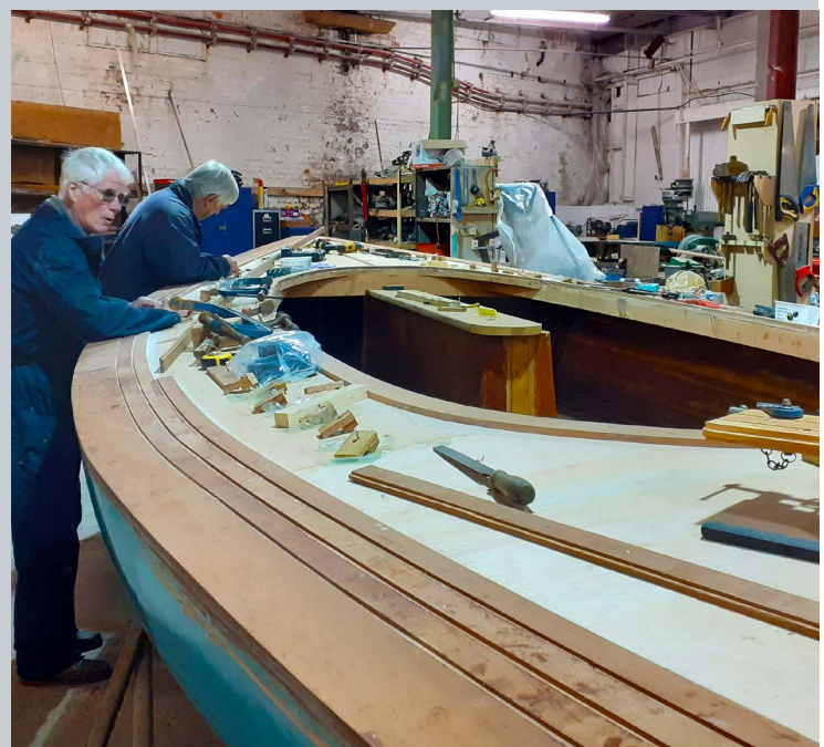
The deck being laid using Gurit AMPRO™ resin.
