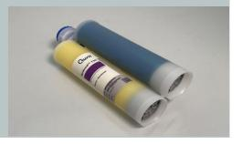
Spabond<sup>™</sup> 730 is a fast curing structural adhesive designed for applications where quick clamp times are important. It has a simple 1:1 by weight and volume mix ratio.
