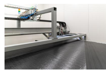
These prepreg stacks are based on Gurit material – either Gurit slit tapes for certified prepreg requirements or Gurit resin taped by Voith for a for maximum production flexibility – both types are manufactured with Voith's VRA NextGen. A Gurit surface layer adds to the outstanding surface quality, making the stacks suitable for visual applications in addition to meeting high structural requirements.
