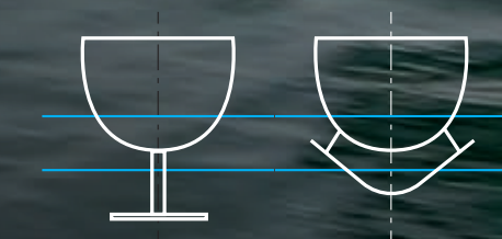
Typical cross section of hydrofoil-supported vessels: Fully submerged (left), Surface piercing (right)
