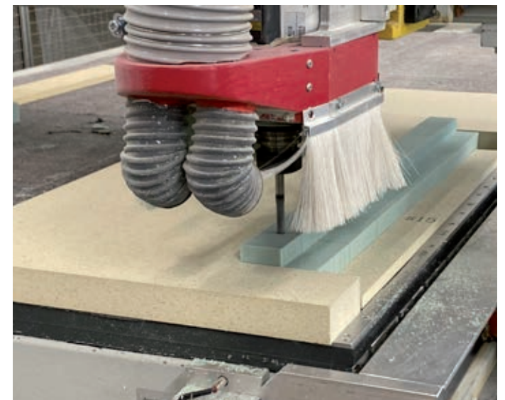
Manufacturing frame extensions from Kerdyn Green PET, Photos courtesy of Geweco-Klebit AG
