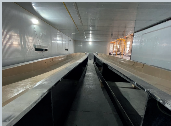
Tooling underway for the 13m hull construction at McConaghy Boats China
