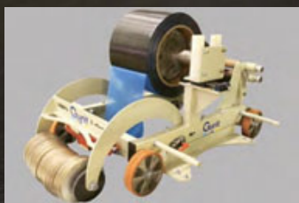
Prepeg laying cart.
