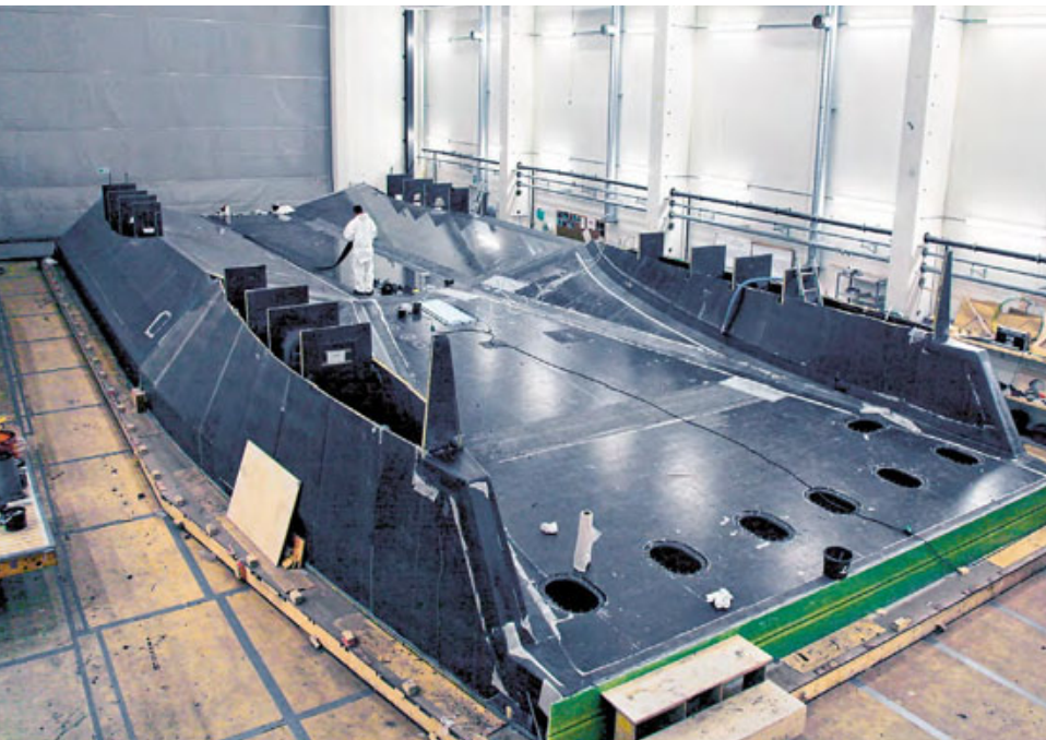
The main deck was infusion-built as one single, very detailed piece and then turned over.
