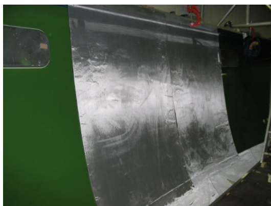
Figure: 2 SF80 Surface Film Application.
