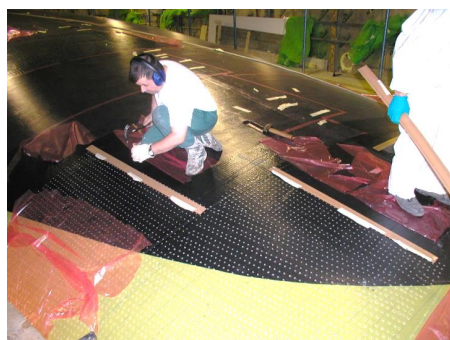
Figure: 6 Spiking Inner Skin to Vent Nomex.
