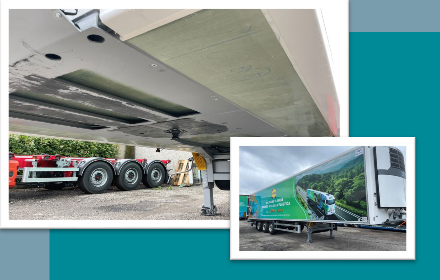
Spanish truck manufacturer Indetruck – The first isothermal trailer with a PET floor, developed for the supermarket chain Lidl.
